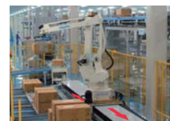
Robot on the shuttle. The robot palletize to multiple locations
